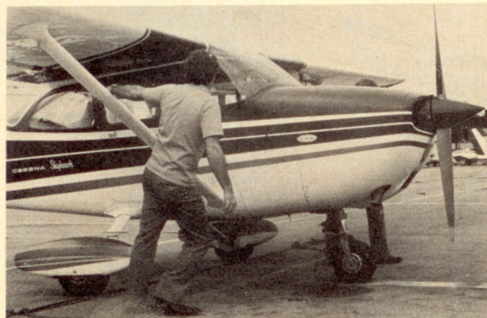
Risking a bent wing strut by pulling on it in mid-span is bad enough, but standing on it to check the fuel tanks is an unforgivable abuse.
