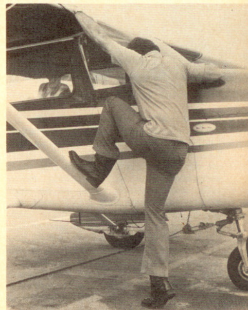
Risking a bent wing strut by pulling on it in mid-span is bad enough, but standing on it to check the fuel tanks is an unforgivable abuse.
